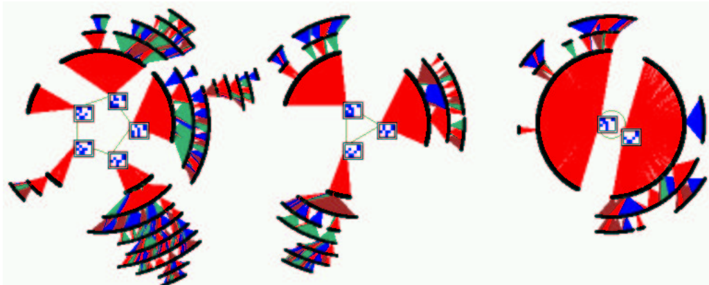
Figure 4: The basin of attraction field of the n=20 sub-network shown in detail in figure 1 ( right ). The rules (input logic) were assigned at random. State-space (size 2^{20} \simeq 1.05 million) is partitioned into three basins of attraction. The attractor states are shown as 5 \times 4 bit patterns. The table and diagram on the right show the probability of jumping between basins due to one-bit perturbations of their attractor states. P = attractor period, J = possible jumps ( P \times n ), and V\% is the basin “volume” as a percentage of state-space. For example in basin 1, P=5 , J=100 possible jumps, 15 of these jump to basin 2, and 85 back to itself, so basin 1 is relatively stable. Basin 3 has relatively few jumps back to itself so is unstable, it is also unreachable from the other basins. The diagram below the table, the “metagraph” (see section 5), shows the same data graphically. Node size reflects basin volume, link thickness percentage jumps, arrows the direction, and the short stubs self-jumps. The fraction of garden-of-Eden states in all three basins is 0.999+ indicating high convergence and order.
