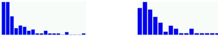
Figure 2: Histograms of link frequency (y axis) against link size (x axis), for inputs+outputs, in the networks in figure 1. The fully connected network ( left ), and modular network ( right ), have a similar link frequency profile. However their dynamics are very different, as described in section 8.
