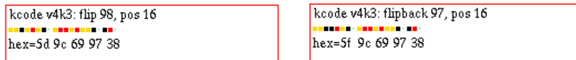
Figure 32.4: Mutating on-the-fly by a random bit/value flip with key 1, restore (flipback) with key 2 — both can be done repeatedly so after multiple flips the original rule can be restored with multiple flipbacks. A top-right window gives information in both cases — this example is for v4k3 kcode, Left : mutation — showing the flip number and its position in the rule-table. Right : undoing the mutation — showing the flipback number and its position in the rule-table.
