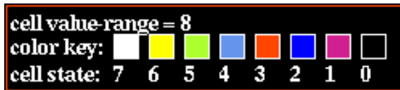
Figure 2.1: The cell value color key window (for a black background, v=8 ) that appears when the value-range is selected. The values themselves are indexed from 7 to 0. See figure 7.1 for all color keys.
