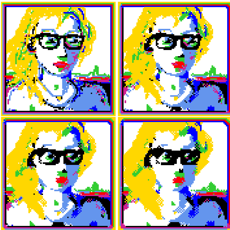
Figure 2.3: Drawing a 2d seed “portrait”, 88 \times 88 , v=8 , with the mouse and keyboard, shown top-left. The seed was then transformed by applying a CA majority rule ( v8k4 ) for three time-steps.
